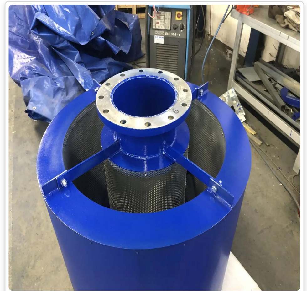
Blue blow-off and start-up silencer with central flange connection
