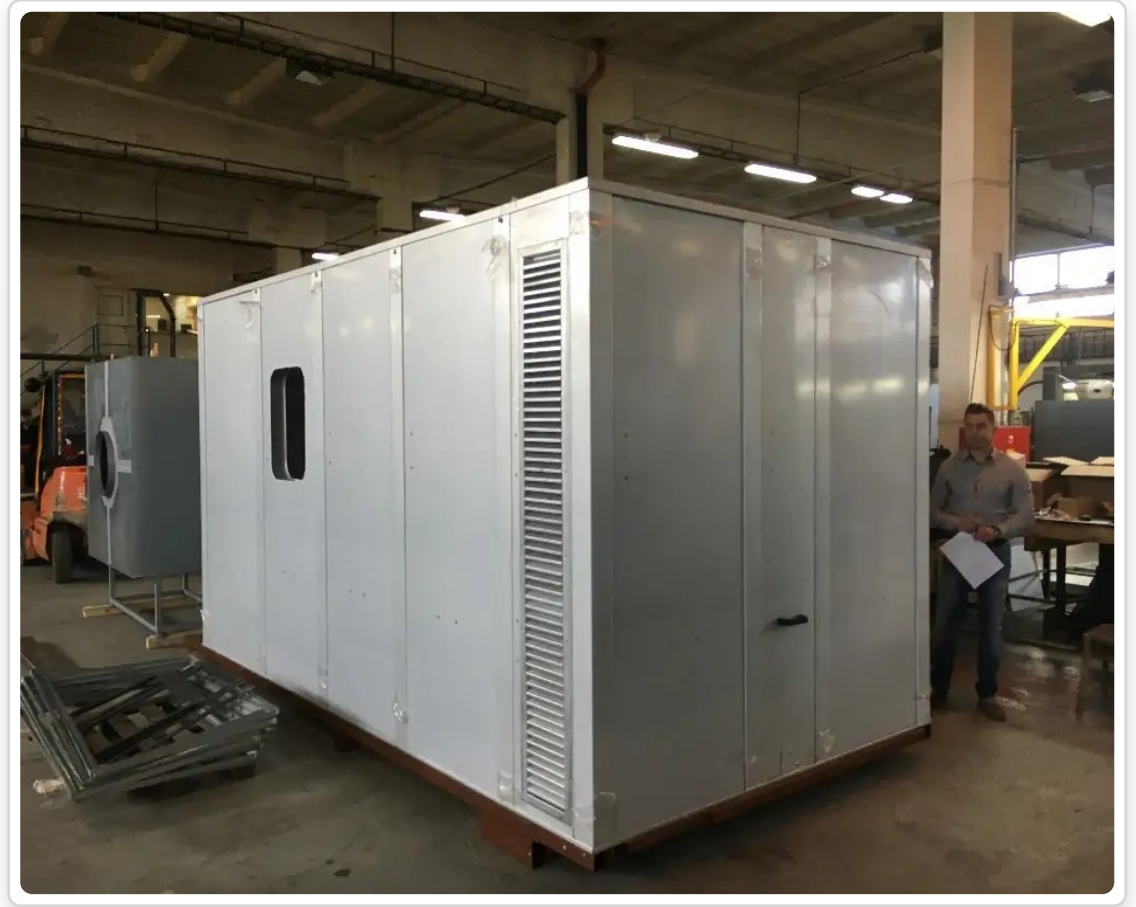
Large modular metal acoustic enclosure for an industrial system in a production hall
